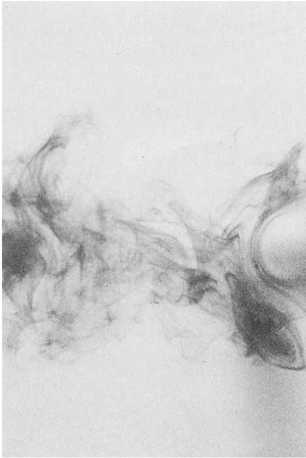
FIGURE 1. A photograph showing plume distortion upstream of the cylinder.
